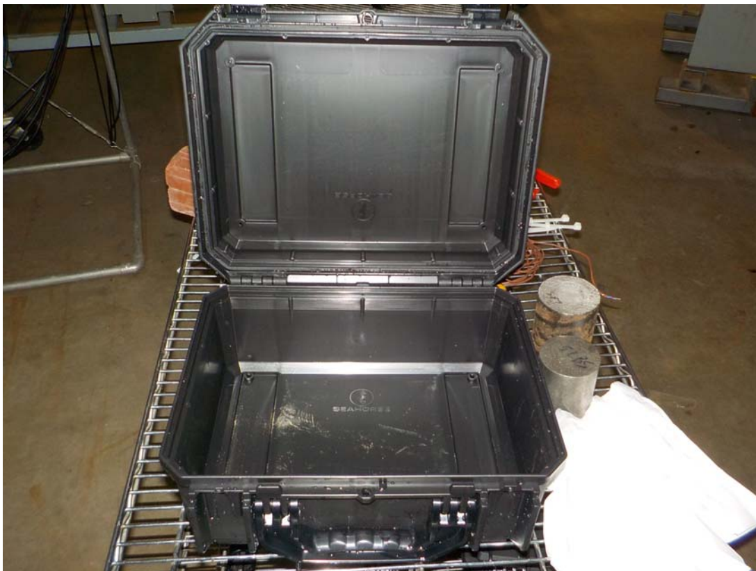
Photograph 4-4: Test unit 58678-3 post-test, no water intrusion is visible
